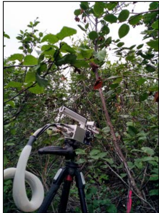
Alders ( Alnus alnobetula ) in thaw slump disturbances are some of the tallest vegetation you will find on the tundra. The instrument pictured (a LI-COR 6400) measures photosynthesis and is being used to investigate whether shrub productivity is higher within disturbances.
